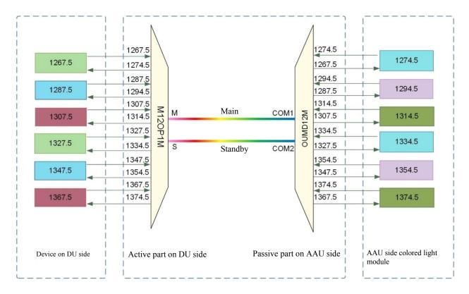
Figure 1-11 Application of M12OP1M board in networking
